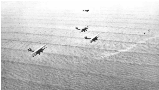
Figure : Aircrafts flying over near-periodic swell in shallow water, close to the Panama coast (1933). The sharp crests and very flat troughs are characteristic for cnoidal waves.
