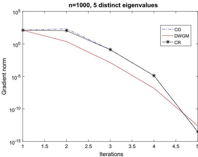
**Fig. 2** Convergence history of DWGM, CG, and CR, from the same initial point, for the minimization of a strictly convex quadratic function, when  $n = 1000$  and the matrix  $A$  has only 5 distinct eigenvalues, equally distributed in the interval  $[10, 1000]$ , each one repeated 200 times
